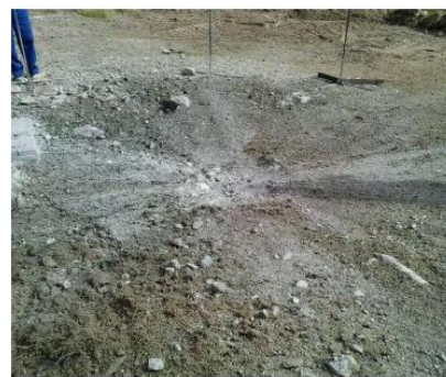
Fig. 5. Detonation of the PBX in contact with the concrete slab [17].
